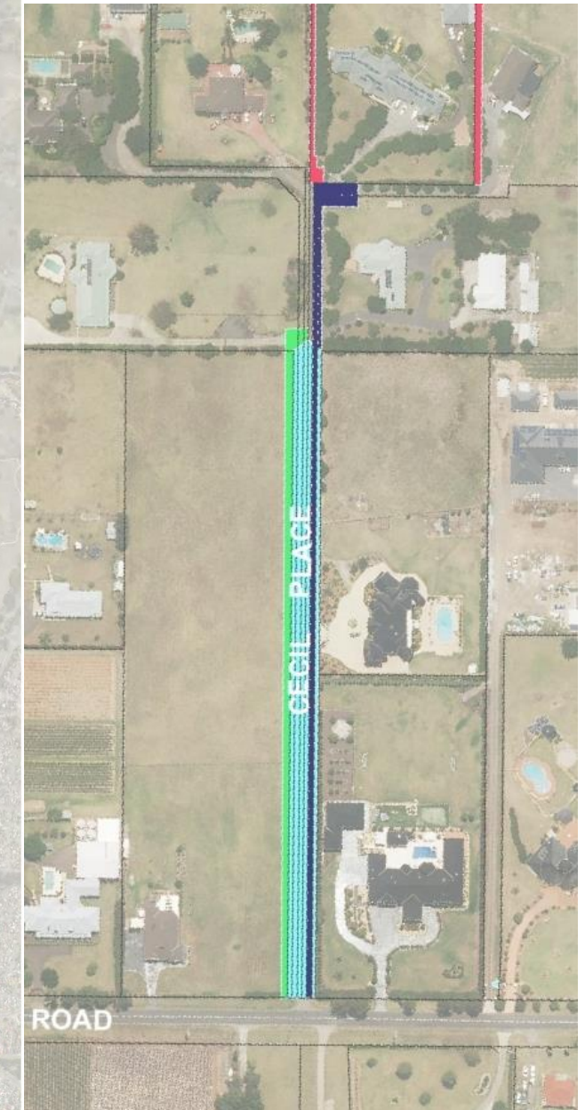
Figure 3-11 Typical access arrangement for battleaxe lots
